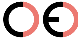
False CE Mark (too far)
